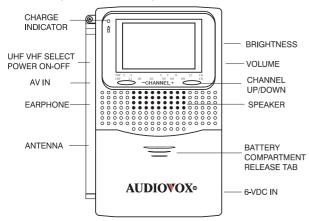
**Charge indicator:**Illumlinates when battreries are charging\* **UHF/VHR Select/Power On/Off:**Turns power on and off;Selects UHF/VHF TV band
